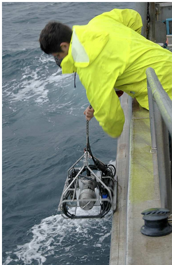
Figure 1: Camera system being lowered over the side of the oyster vessel Polaris .
